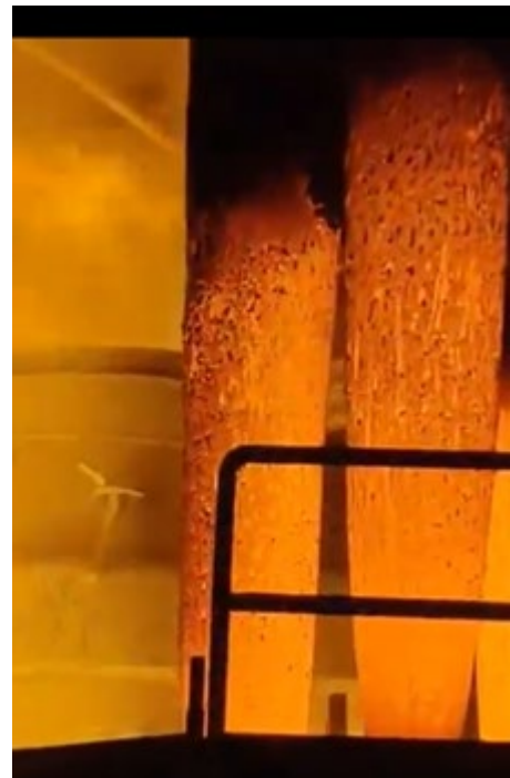
Figure 2 / Lateral burning of the electrodes
