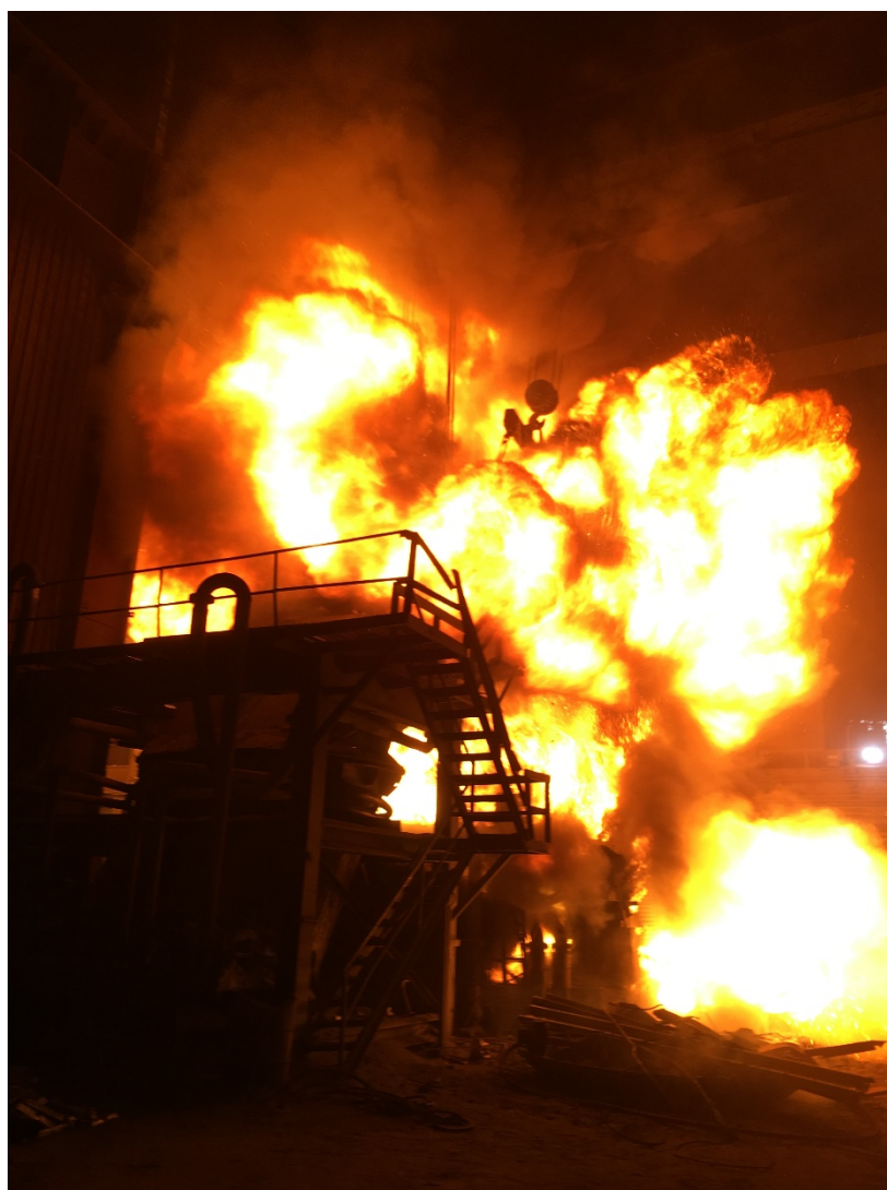
Figure 2 / Massive fire when scrap charging as pollutants are firing-off
