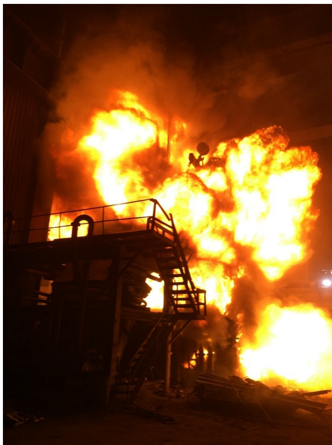
Figure 4 / chemical reactions when charging scrap into an open furnace
